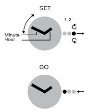
To set the time, pull the crown to position 2. Turn slowly to correct minutes. Turn quickly to correct hours. After resetting has been completed, push the crown back.
